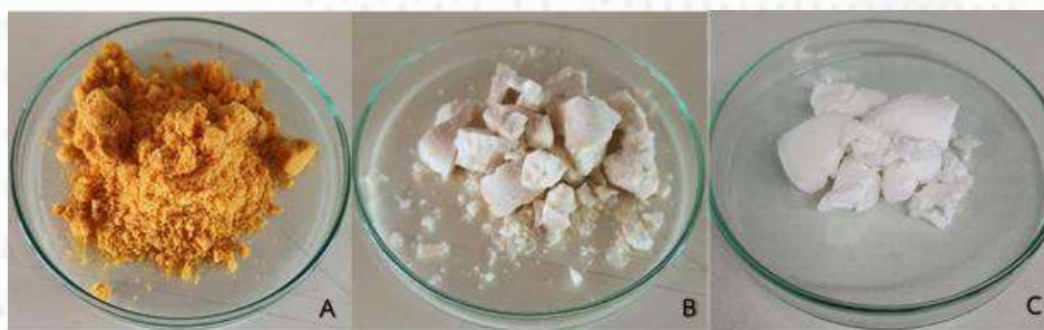
ภาพที่ 1. The microcapsule of essential oil from the seed of O. gratissimum with different encapsulation substances (shell) A) WPI, B) GA, and C) PVA.
